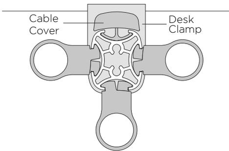
**8.4** To reposition the cable cover, pull it straight up and out of the post and insert it into any of the available channels
