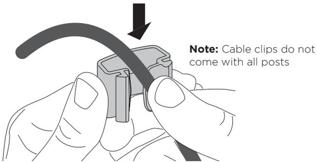
**8.2** Push cable clip into post channel
