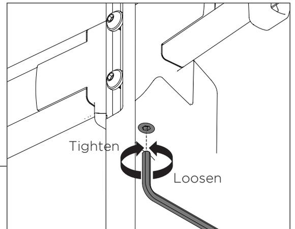
**OPTIONAL** If the crossbar rotation is too loose or stiff, adjust the tension screw under the centre of the crossbar.
