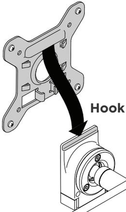
**4.2** Gently push the bottom of the monitor until the VESA plate locks into place.
