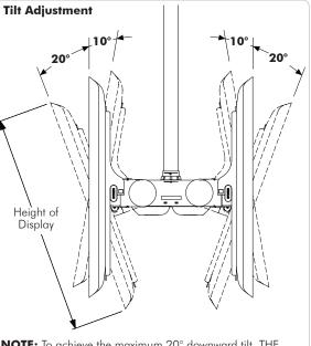
**NOTE:** To achieve the maximum 20° downward tilt, THE MAXIMUM HEIGHT OF A DISPLAY IS 1143mm (45"). NB:For Displays greater than 1143mm, there will be a reduction in the achievable tilt angle.
