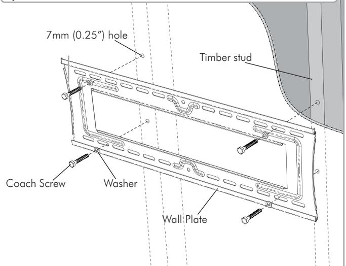
**TIP:** Use a spirit level to ensure the wall plate is horizontal
