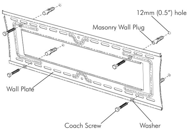
**TIP:** Use a spirit level to ensure the wall plate is horizontal
