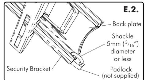
For additional security, it is suggested that a Padlock is attached through the Security Bracket and the Wall Plate on either side as shown. The Padlock (not supplied) should have a shackle diameter no larger than 5mm ( $\frac{3}{16}$ ").
