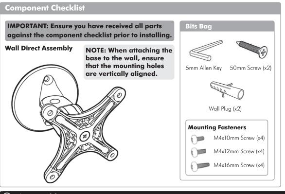
Focus Wall Direct supports a maximum weight of 8kgs (17.5lbs)
